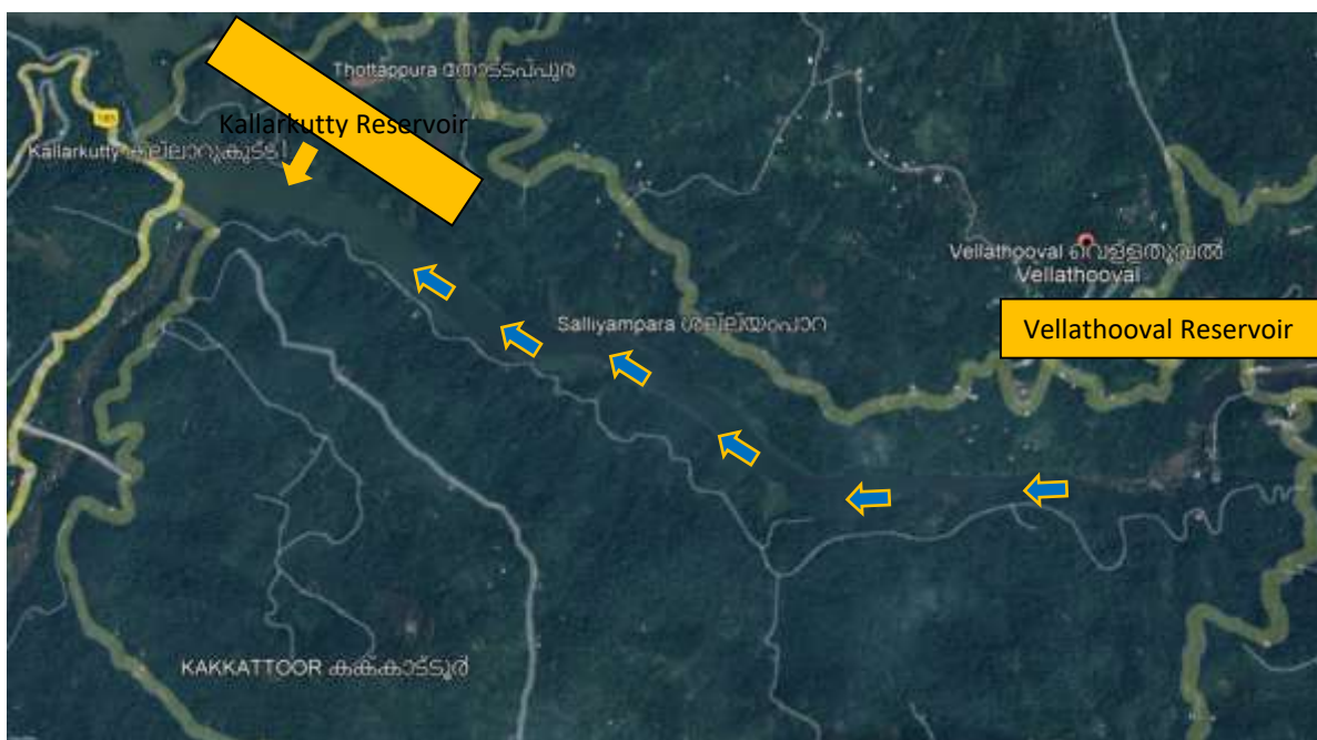
Fig 1.10: Flow path of spill water
